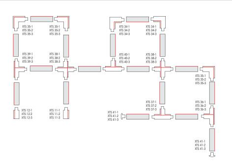
Diagram above shows the use of L-, T- and X- Feed. Red line marks the polarity ridge. Available colours: –1 grey (RAL 7040), –2 black (RAL 9005), –3 white (RAL 9016).
